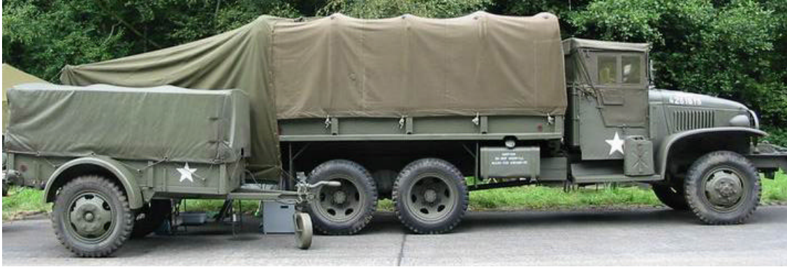
GMC 2.5 ton CCKW Prime Mover for 105-mm Howitzer – WWII, soft cab version
